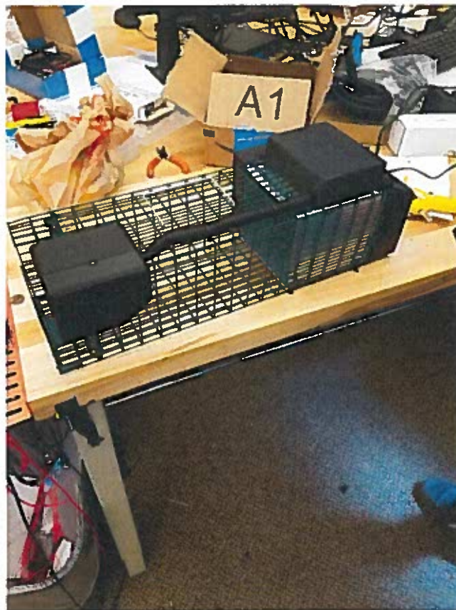
Figure 2: The NEMA 17 motor and gears at the front of the trap are shielded by a 3D printed cover.
